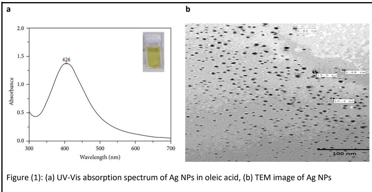
Figure (1): (a) UV-Vis absorption spectrum of Ag NPs in oleic acid, (b) TEM image of Ag NPs
